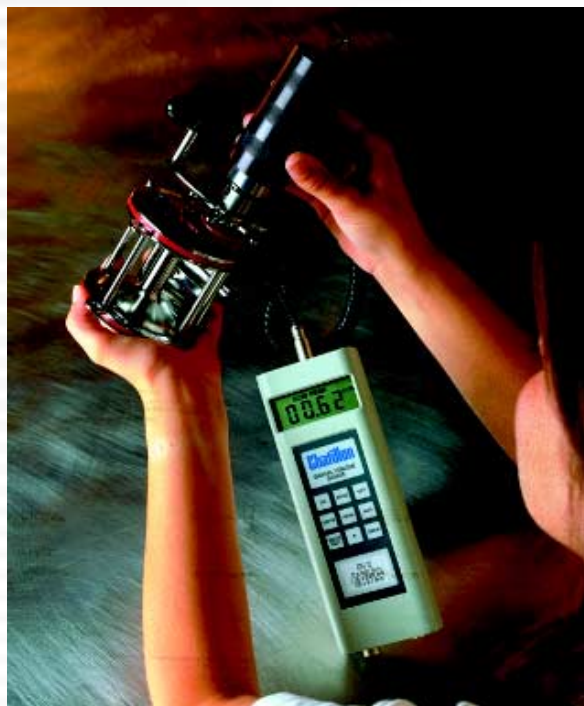
DTG measuring fishing reel torque
